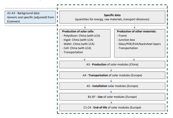
The PolySi, ingots, wafers, cells and modules are manufactured in China. The supply chain is shown below:
