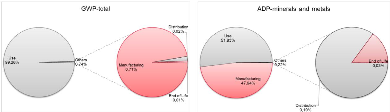
Figure 5 Contribution analysis for the average mineral oil transformer
