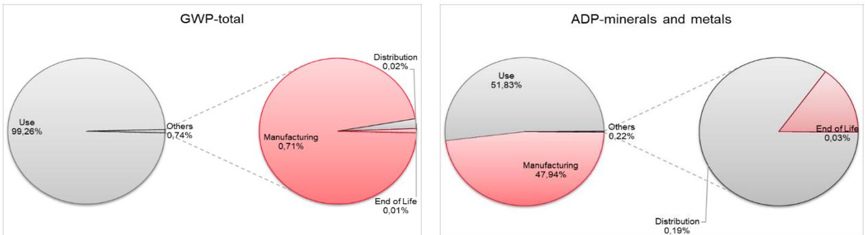
Figure 6 Contribution analysis for the average natural ester oil transformer
