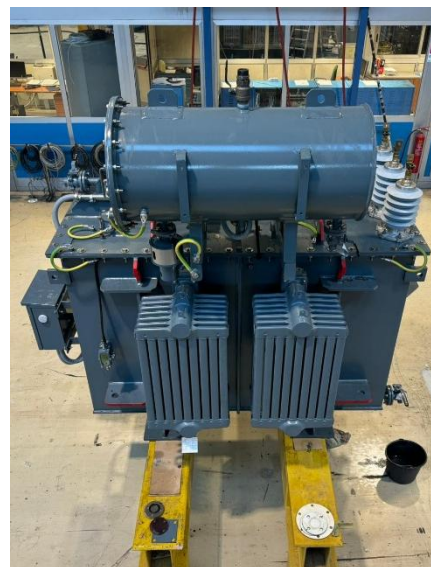
ATR MT/MT 6 MVA 20/15kV
