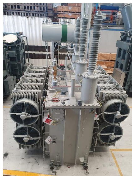
TR 40MVA 115/12KV OLTC NATURAL ESTER
