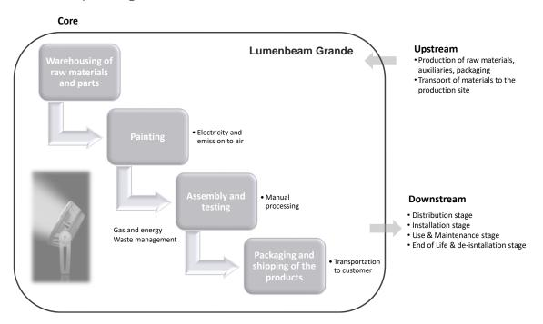
All input and output flows are inventoried for each stage of the life cycle. Flows, materials and energy extracted from the environment and released into it are then combined at each stage to quantify environmental impact indicators.
