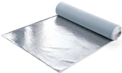
Elotene DSFR 800 is a self-adhesive bituminous waterproofing membrane that forms a total barrier against vapour. It consists of a specific fire-retardant compound (calorific value < 10.500 kJ/sqm) self-protected by a reinforced aluminium foil and a fibreglass net, which guarantees high mechanical performance. It is particularly indicated for industrial metal deck applications. The membrane complies with DIN 18234. Thickness 0,4 mm.
