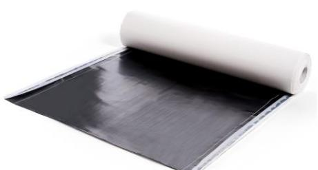
Elotene 3000 X is a self-adhesive bituminous waterproofing membrane self-protected by a cross-laminated HDPE film. The high-density polyethylene film gives to the membrane characteristics of dimensional stability and ensures a uniform reaction to elongation stresses in a longitudinal and transversal direction. Thickness 1.5 mm.
