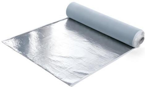
Elotene DSN 800 is a self-adhesive bituminous waterproofing membrane that forms a total barrier against vapour. The product consists of a self-adhesive low-thickness bituminous compound, self-protected by a reinforced aluminium foil and a fibreglass net. The so composed film makes the membrane resistant to heavy worksite traffic and suitable for applications that involve high mechanical stresses. Thickness 0,6 mm.
