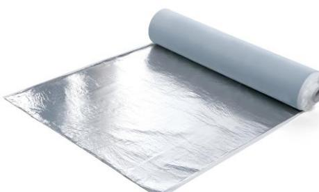
Elotene DS is a self-adhesive bituminous waterproofing membrane that forms a total barrier against water vapour. It consists of a self-adhesive and self-sealing bituminous compound with a reinforced aluminium film on the surface. The polyester reinforced aluminium makes the membrane resistant to work site traffic. The product is not affected at all by ageing and is compatible with most of construction and industrial materials. Thickness 1,2 mm.
