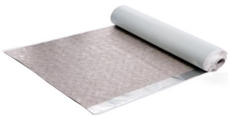
Elotene DSR is a self-adhesive bituminous waterproofing membrane with a skid inhibiting surface that makes it ideal as carrier membrane in multilayer systems. It consists of a self-adhesive bituminous compound self protected with a reinforced aluminium foil and a non-woven skid inhibiting layer. Thickness 1,2 mm.
