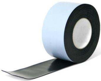
Elotene TUBI V7 bitumen compound is a self-adhesive tape made of a soft adhesive bitumen compound protected by a thin HDPE film. The tape is designed for applications that require excellent malleability. Thickness 1,5 mm.
